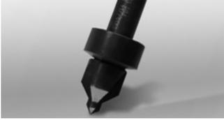
Due to the material-dependent expansion of the Rhenoplast transparent panels, depending on the panel length, corresponding holes must be predrilled into the panels (see also our Rhenoplast installation instructions). The special Rhenoplast drill bits fitting any standard drill chuck are available in three sizes: diameter 10, 12 or 14 mm.
